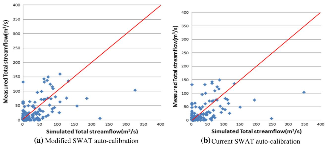
**Fig. 7** Comparison of low flows of current and modified auto-calibration
